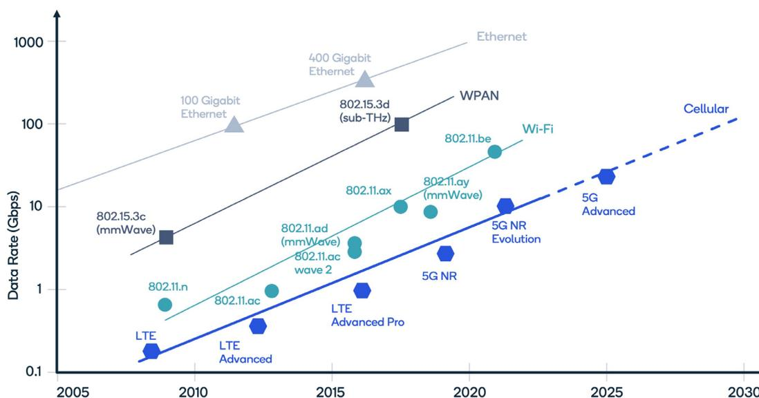
Figure 24: Growth of data rate in communication standards
